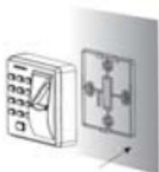
(4) Fix the device to the back cover.
