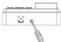
(1) Remove the screw on the bottom of device.
